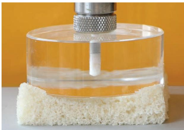
For this purpose, all loaves were measured 24 and 72 hours after baking using Texture Analyzer Brookfield CT3 (see figure 2). The loaves were measured using the same method of sample preparation and measurement parameters. Hardness was calculated and compared. Hardness increase over time is a textural attribute related to ageing of bread (Demirkesen et al., 2013).<sup>[4]</sup>
